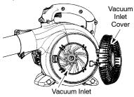
Align the tabs on the inside of the vacuum in-4. let with the slots on the upper vacuum tube.
